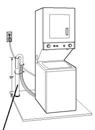
Standpipe drain system: Needs a two-inch minimum diameter standpipe with minimum carry-away capacity of 17 gallons per minute. Top of standpipe must be at least 39 inches above floor and no higher than 96 inches from bottom of laundry center.
